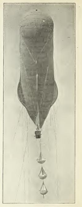
Fig. 25. Head-On View of Modern Kite Balloon, Showing Details of Tail Buckets Copyright by Central News Service, New York City
