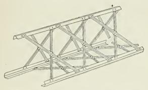
Fig. 17. Trellis Type of Aluminum Girder used in Longitudinals of Zeppelin Frame
